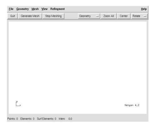
It consists of the menuline and the button line at the top, the status line at the bottom, and the large drawing window. The menu items will be explained in 6.1. The button line provides shot-cuts for common opteration:
